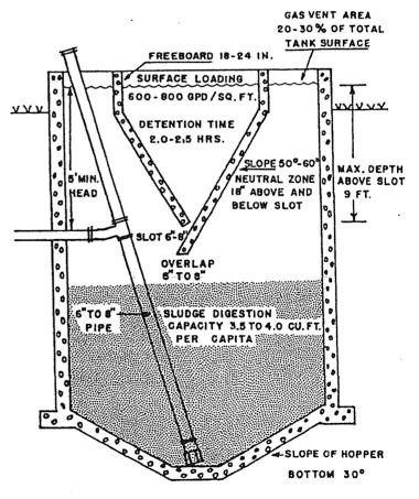
Figure 2. – Cross-section of Imhoff
