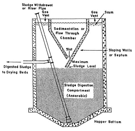
Figure 1. – Cross-section of Imhoff
