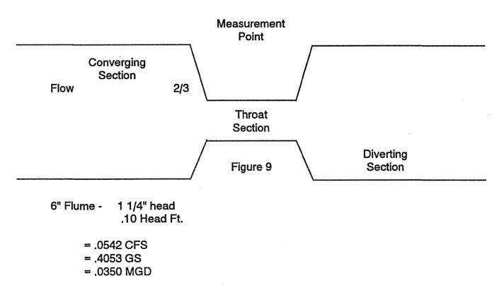
To obtain an accurate flow measurement of a flume, you must measure the head and know the width of the throat of the flume.
