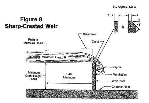
head = 16" upstream of weir crest to take measurement. Go to chart (lsco) and find actual flow measurement.
