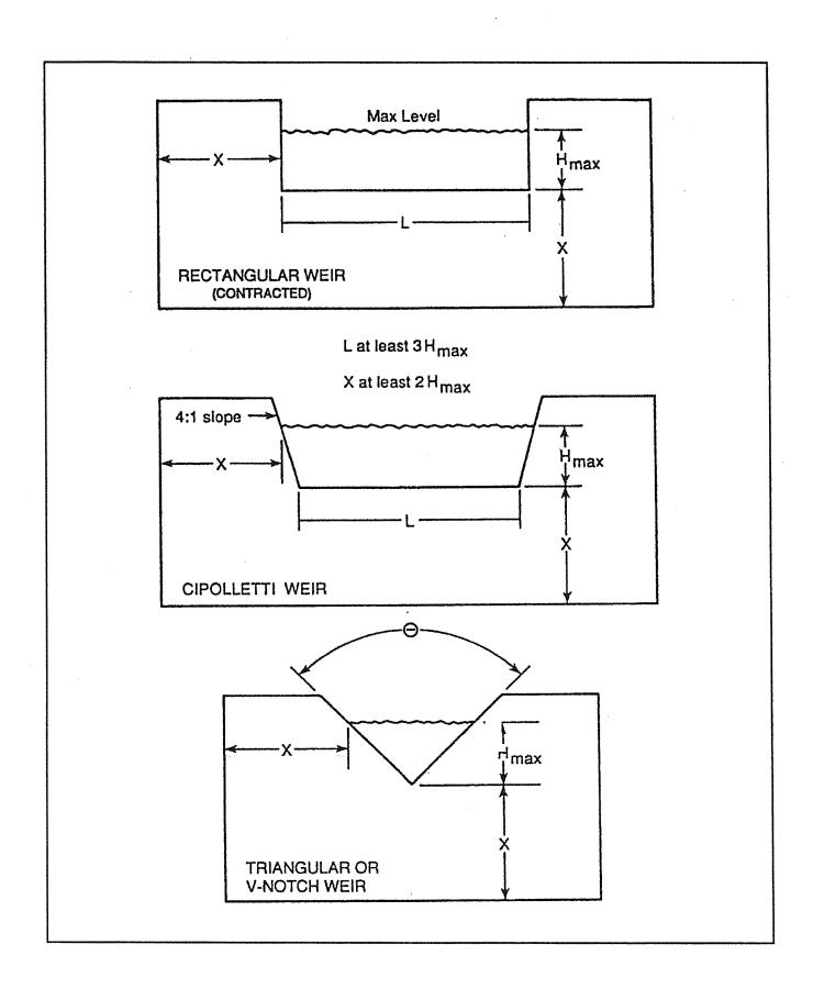
Figure 7. – Three Common Types of Sharp-Crested Weirs
